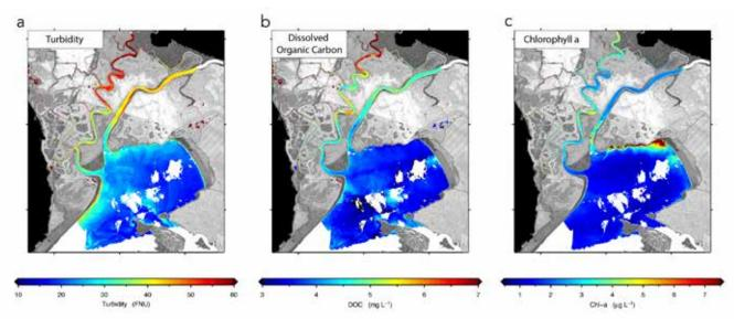
**Figure 33.** Maps of (a) turbidity (water clarity), (b) dissolved organic carbon, and (c) chlorophyll-a in the San Francisco Bay-Delta Estuary's Grizzly Bay and Suisun Marsh in April 2014, derived from remote-sensing reflectance data from NASA's airborne Portable Remote Imaging Spectrometer (PRISM) instrument. Source: NASA/JPL-Caltech (2016).
