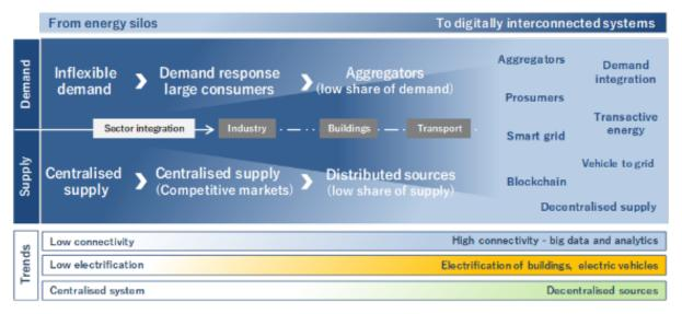
**Figure 25.** Possible steps in the digital transformation of the electricity system. The deployment of digital technologies is creating a more interconnected and responsive electricity system, with the potential to help increase flexibility, efficiency, and reliability. Source: IEA (2017).
